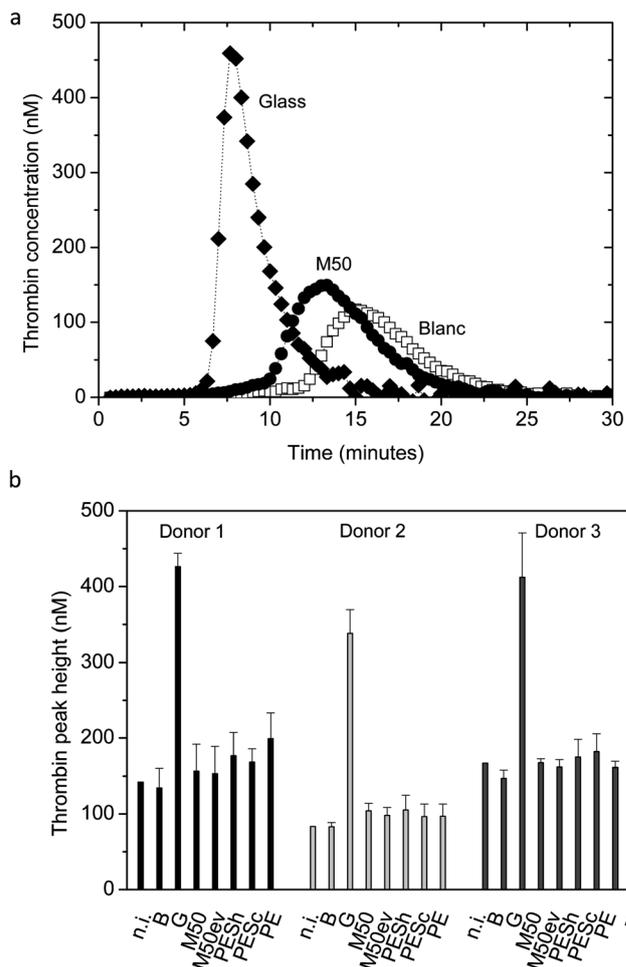
**Fig. 4** (a) Typical thrombin generation curve for blank (incubated PPP) ( $\square$ ), glass ( $\blacklozenge$ ) and a M50 membrane ( $\bullet$ ). (b) Average thrombin peak height presented for the categories: n.i. (not incubated PPP), B (blank, incubated PPP), glass, M50, M50ev, PESh, PEsc and PE for donors 1, 2, and 3. Error bars indicate standard deviations.
