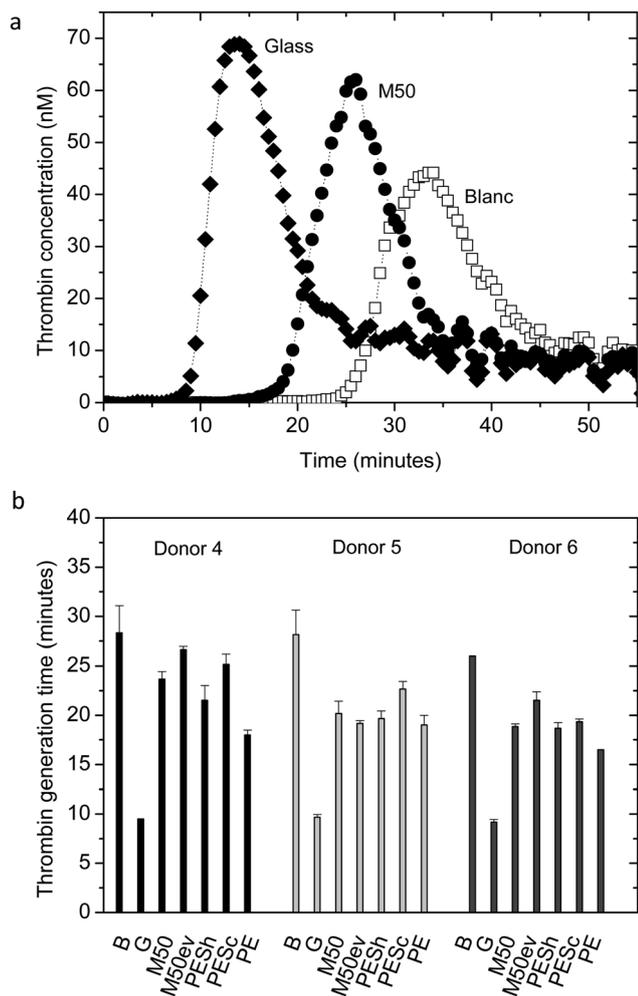
**Fig. 5** (a) Typical thrombin generation curve of glass (◆), M50 (●) and blank (incubated PRP) (□). (b) Average thrombin generation times presented for donors 4, 5, and 6, for the following materials: B (blank, incubated PRP), G (glass), M50, M50ev, ESh, PESc, PE membranes. Error bars indicate standard deviations. Thrombin generation times were measured in triplicate for each material and each donor.
